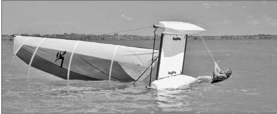
Figure 11-10: Using a righting line to add leverage and right a capsized catamaran.
