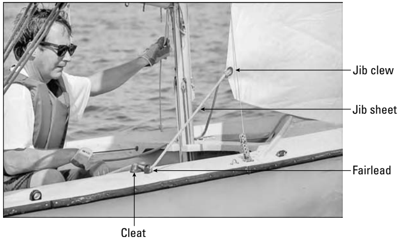
Figure 4-11: Jib sheet system on a 420-class dinghy.
