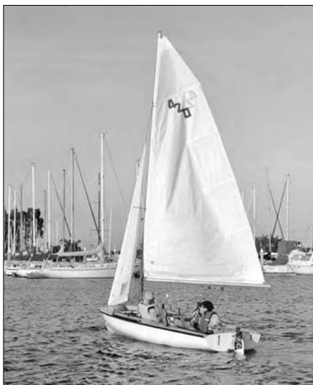
Figure 14-3: Heaving-to: Cleat the jib on the windward side and let the main luff. Now you can take a break.
